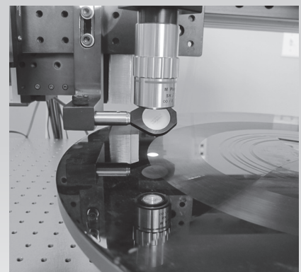
IRENE's 2D camera images the grooves on a lacquer disc.
